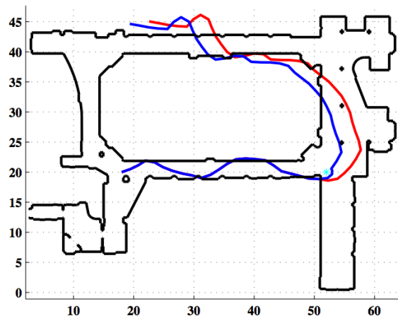
(b) Paths estimated by PDR (red) and path corrected (blue) by 1 tag (cyan star).
