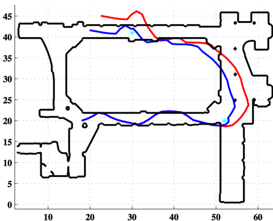
(c) Path estimated by PDR (red) and path corrected (blue) by 2 tags (cyan stars).
