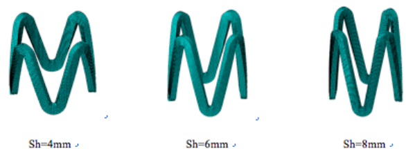
Fig. 5. Finite element computational grid model for annular supports with different widths.
