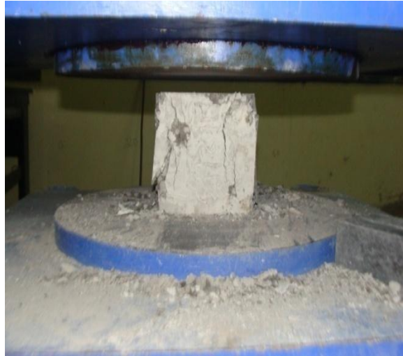
Plate 5. Test set up of cube compressive strength
