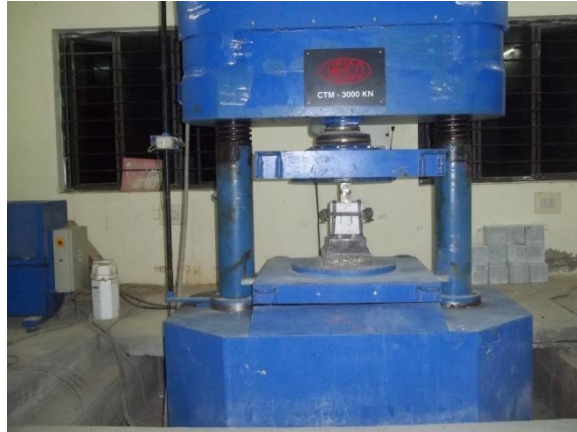
Plate 7. Test set up of dcn cubes
