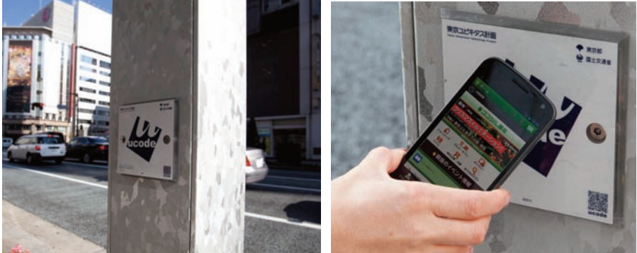
Figure 11 - (left) Tag along Ginza street, (right) Reading it with a mobile phone with NFC tag reader
