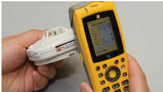
Figure 12 - Smoke detectors are scanned to record the installation place and date
