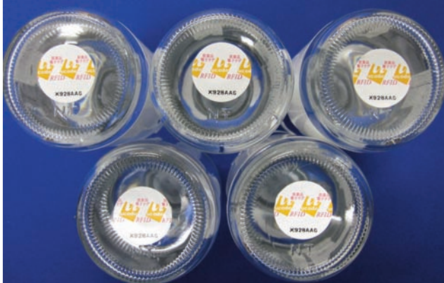
Figure 13 - Tracking drug bottles by RFID tags on the bottom
