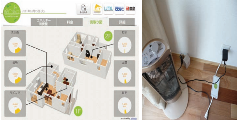
Figure 6 - (left) Monitoring of electricity usage at home, (right) Smart Meters in a room
