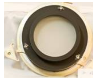
Fig 10 : Diffuser monitoring (internal side)
