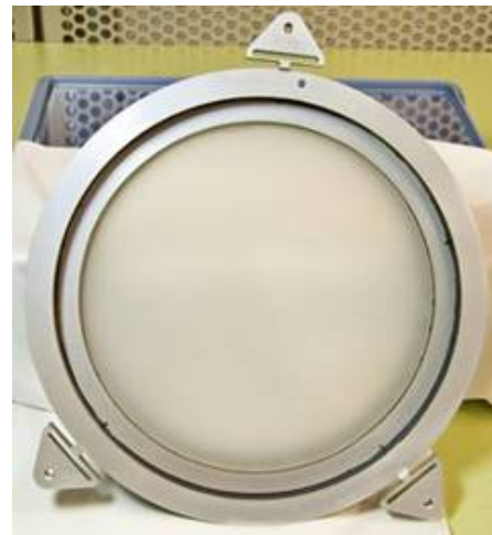
Fig 9 : Full pupil Solar Diffuser (external side)
