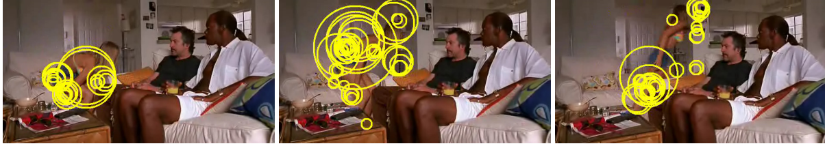
Figure 2. Space-time interest points detected for multiple video resolutions and three frames of a StandUp action. The circles indicate spatial locations and scales of space-time patches used to construct bag-of-features video representation (see text for more details).
