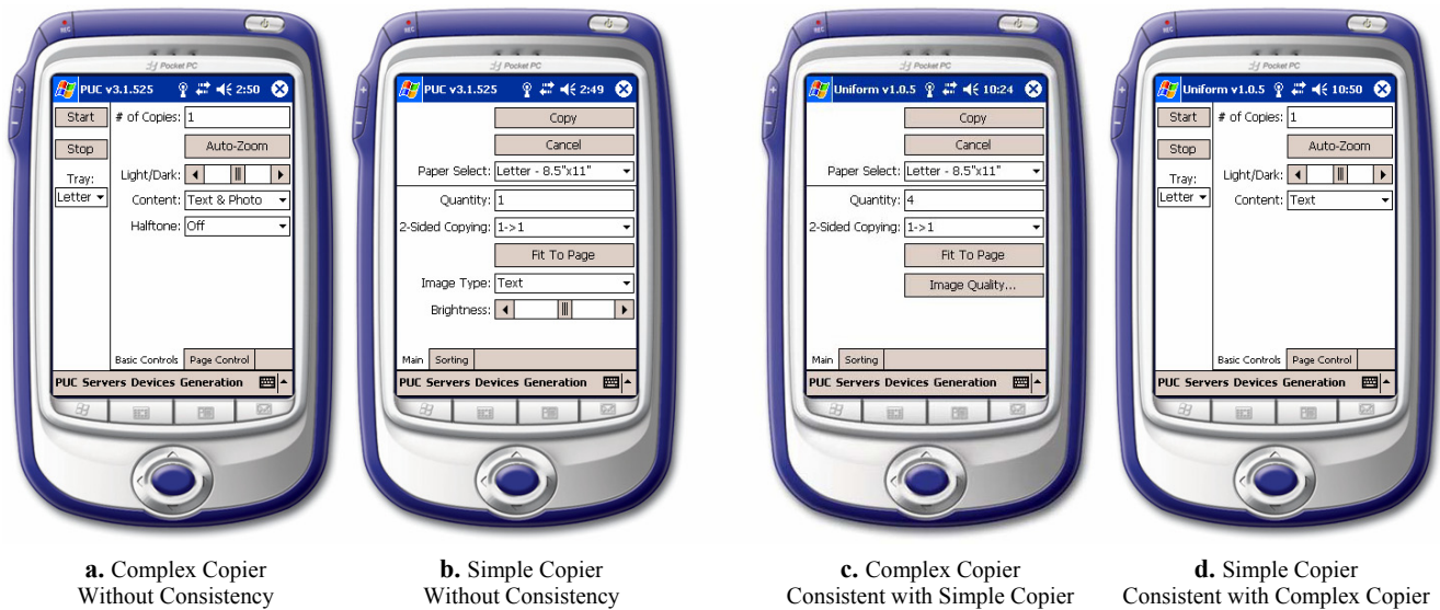
Figure 1. User interfaces generated by Uniform for a complex and simple copier without and with consistency.
