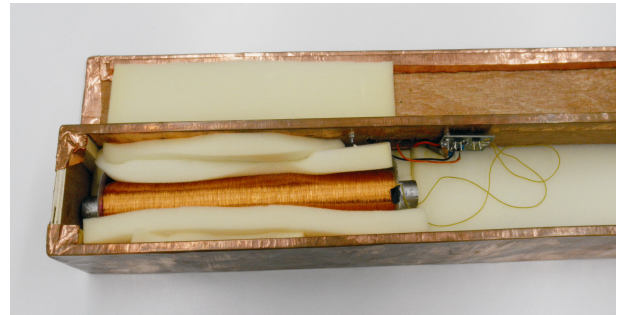
Fig.1. Installation of the inductor coil
