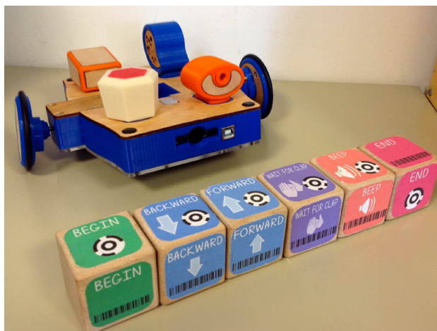
Figure 1 KIWI Robot and CHERP Programming Blocks
