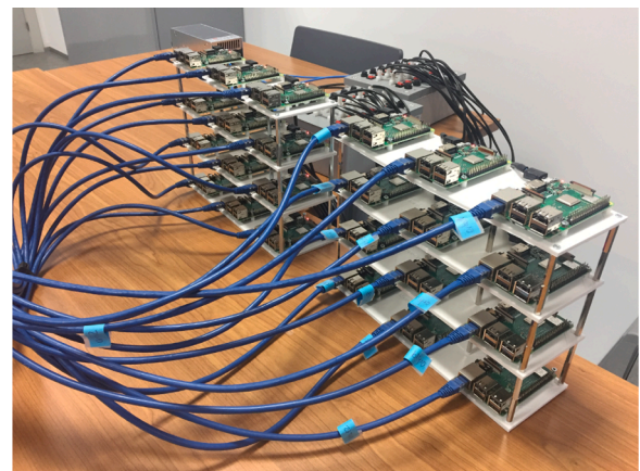
Fig. 7. Raspberry Pi cluster used as Fog infrastructure in the SHM architecture.
