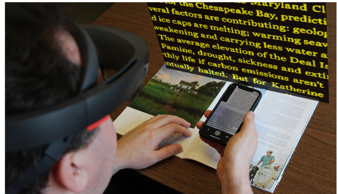
Figure 1. Prototype AR Magnification system using a transparent HMD (the Microsoft HoloLens) and a handheld smartphone (iPhone X) as a camera and input device.
