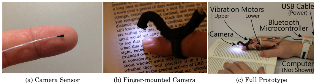
Figure 1: HandSight uses a 1\times 1\text{mm}^2 AWAIBA NanEye 2C camera developed for minimally invasive surgeries (e.g., endoscopies) that can capture 250\times 250\text{px} images at 44fps (a). Also shown are two early designs for our finger-based reading system (b) and (c). Future designs can be made much smaller.
