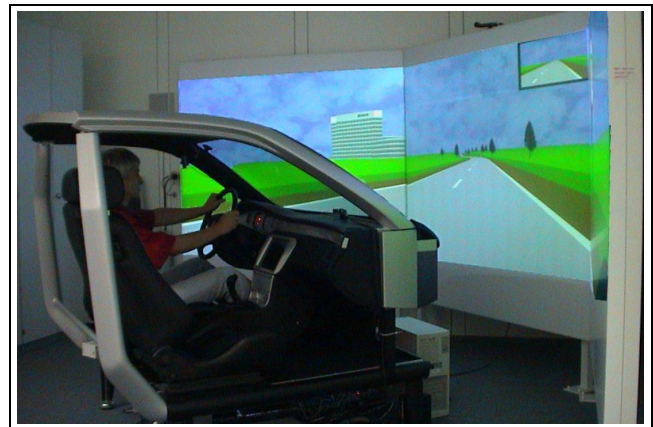
Figure 1: View of the Bosch driving simulator
