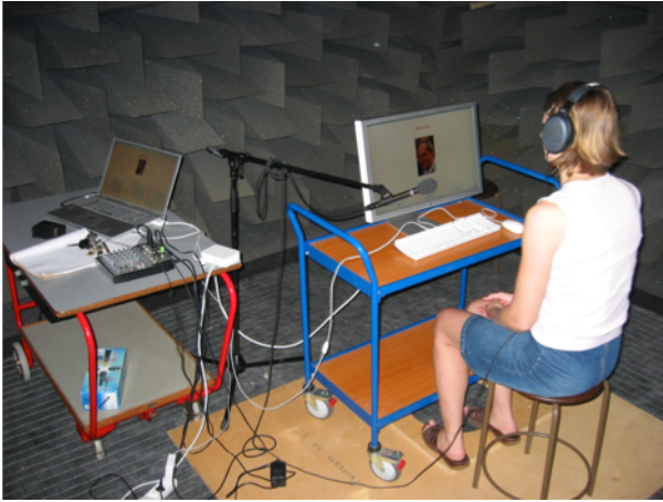
Figure 5 Recordings for Y2 Finnish took place in an anechoic chamber. A technician was seated by the table on the left controlling the issuing of prompts for the speaker as well as monitoring all recordings for accuracy and quality of elicitation.
