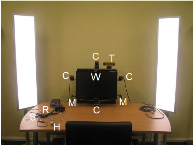
Figure 2: The hardware setting in the subject room. C=High resolution camera, H=Heart beat clip, M=Microphone, R=Respiration belt, S=Skin conductance clip, T=Stereo camera, W=Observation webcam. Not in the picture: Headwear microphone.
