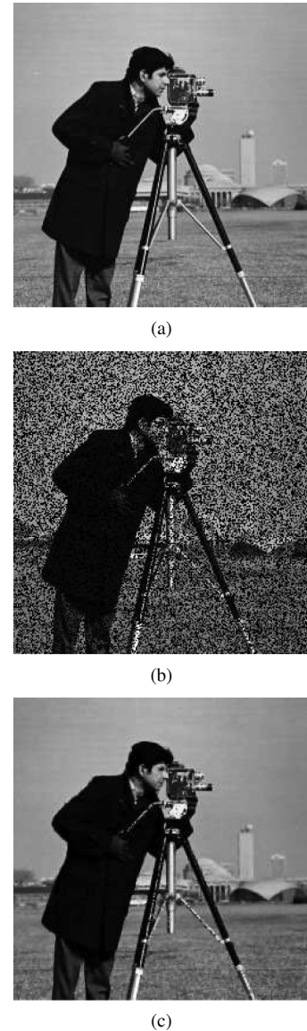
Fig. 6. Image inpainting with TV regularization: (a) original cameraman image; (b) image with 40% pixels missing; (c) estimated using SALSA.
