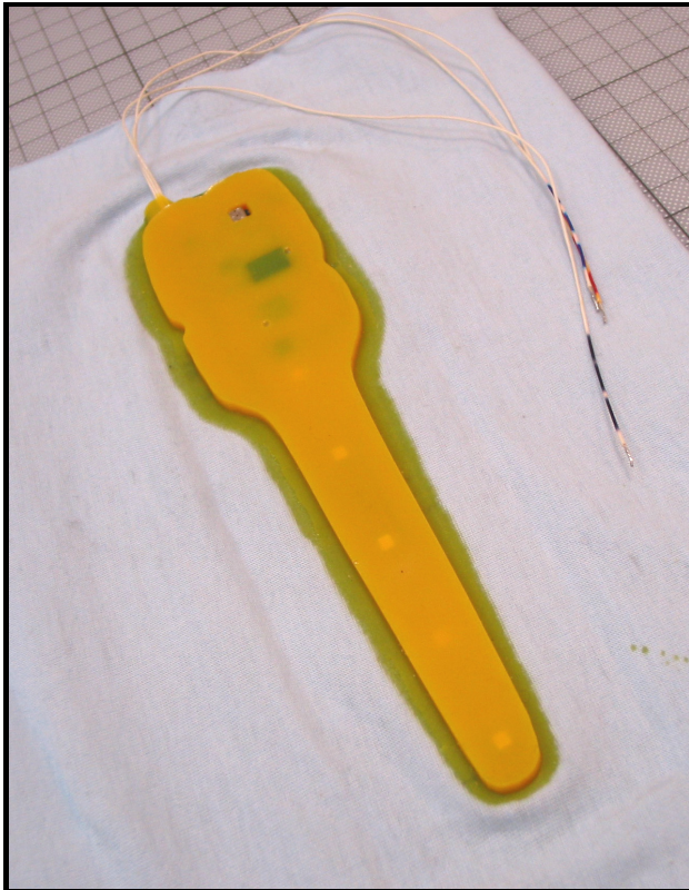
Fig. 2. Open-cast machine-washable, flexible, polymer-cast circuit board. Note the microphone in the cavity.
