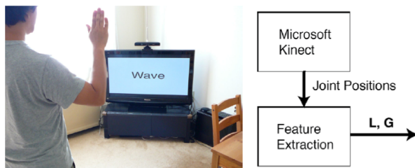
(a) User in front of display and Kinect executing a wave gesture (b) Extraction of feature vectors from Kinect images
