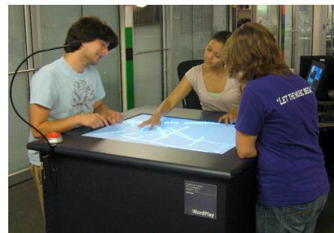
Fig. 3. WordPlay table with microphone and voice recognition as input device for idea generation. Manipulation and organization of displayed phrases via touch gestures [10].
