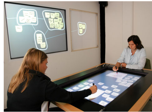
Fig. 2. Idea generation and organization with the table and wall setup. Post-its are created and organized with a pen. The wall display is used for categorization and overview [9].
