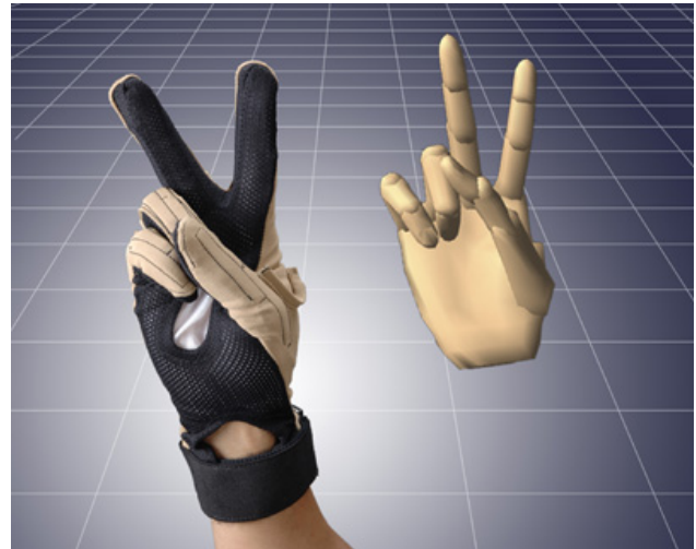
Fig. 2: Example for an invasive sensing device: the CyberGlove [7]
