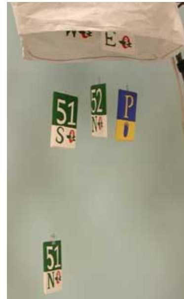
Fig. 2. Image of the BusMobile Ambient Information System [8]. It displays bus departure times from a nearby terminal. The time frame roughly corresponds with the distance to the top.
