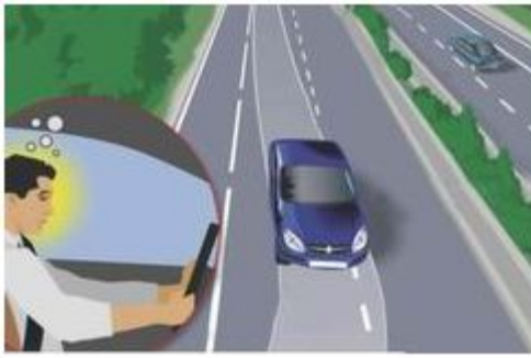
Fig. 5. The Lane Departure Warning System warns the driver by a vibrating mechanism in the seat if he crosses the lane, for example because of fatigue or negligence [20].
