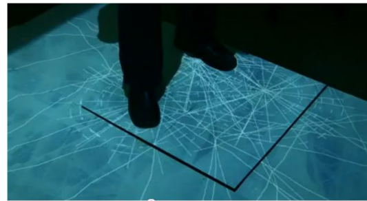
Fig. 10. A haptic floor that simulates a frozen lake. The user not only sees but also feels the cracking of the ice if he steps to hard [14].
