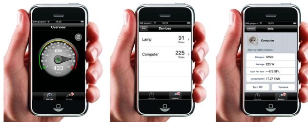
Fig. 6. The mobile user interface shows the current entire consumption of all devices attached (left), a list of discovered Ploggs including their name (middle), and more detailed information per Plogg (right) [29]
