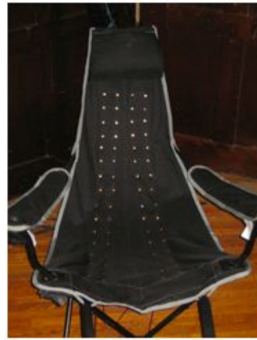
Fig. 4. A haptic chair as a sensory substitution system. The music chair enables deaf people to hear music by converting sound into vibrations [24].
