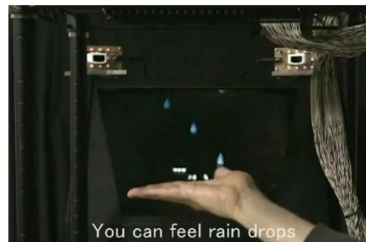
Fig. 11. Airborne Ultrasound provides tactile feedback to the users hand in 3D space. For example it can enable the user to feel rain drops on his hand that are displayed on a screen [21].
