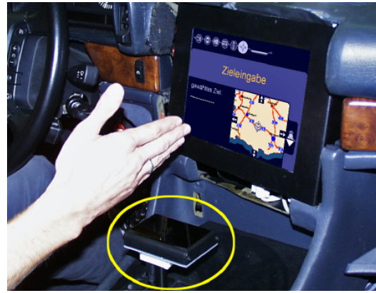
Fig. 6: Integrated GeCom system with IR sensor array (yellow) [10]
