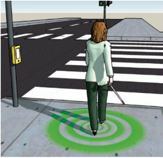
Fig. 3. A haptic floor that helps blind people in the road traffic. Vibrotactile cues provide information whether the crossing signal is red or green [26].
