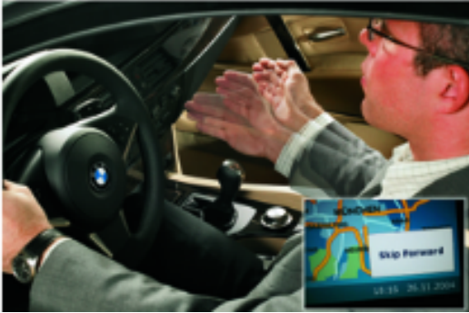
Fig. 8. Control of the CD-player: waving to skip between songs [3]
