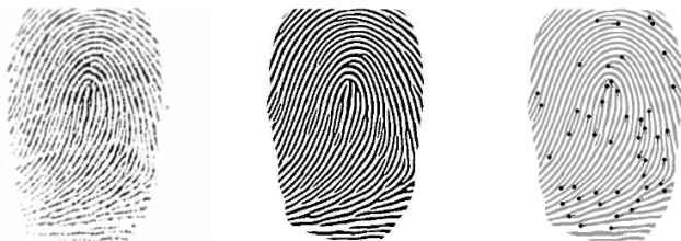
Fig. 4. Fingerprint feature extraction: (a) original image, (b) edge detection, (c) feature points (minutiae) [14]
