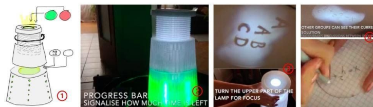
Figure 1. stayFOCUSed experience prototype (1. Prototype structure; 2. Progress bar in traffic light; 3. Rotate the projector to show answers; 4. Hand-write in the disk)
