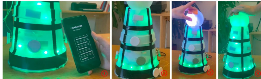
Figure 3. Tower experience prototype (1. Discuss with other groups through App; 2. Place magnets on the Tower to choose an answer, green is "I'm confident", white is "I'm not sure"; 3. Rotate top bulb for help; 4. Touch top bulb to show finished)
