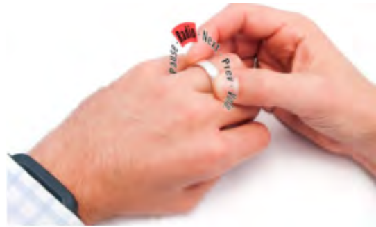
Fig. 10. Ashbrook et al. suggest input via a discrete, magnetically tracked finger ring and a wrist-mounted sensor [1].
