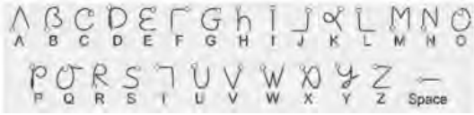
Fig. 6. The Graffiti alphabet is a stroke based alphabet which is easy to learn for novices due to its strong resemblance to the roman alphabet [17].
