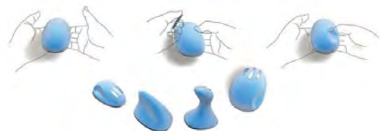
Fig. 2. Moldable mouse of jelly-like material [Lite-On, 2007].
