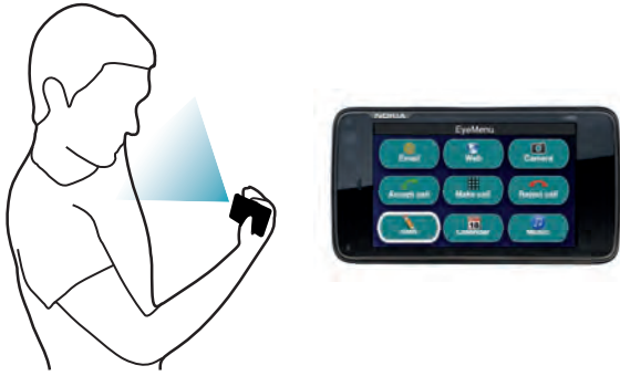
Fig. 6. EyePhone: Controlling the interface with eyes only [24].
