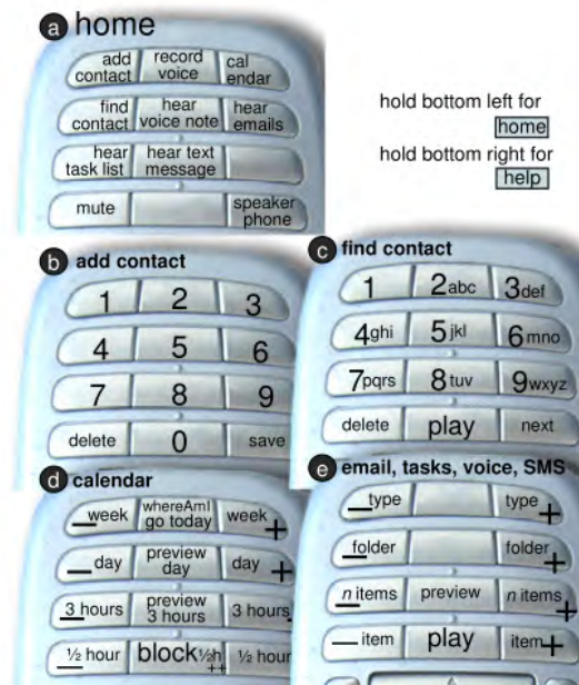
Fig. 5. BlindSight's menu structure. a, b and c use the menu pattern: A small number of different choices can be accessed directly by pressing the corresponding button. d and e use the iterator pattern, which allows iterating through a list of choices. [10]
