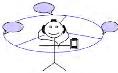
Fig. 1. Brewster et. al. developed a 3D auditory radial pie menu, in which the user is centered. Menu items are represented either by speech or by sounds and are situated around the user. Each menu item is selected by nodding the head in the direction, the sound is coming from.[5]
