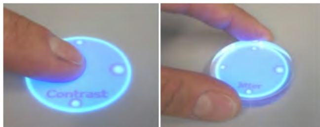
Fig. 5: An "effect" object rendered as a digital object on the surface (left) or overlaid with a piece of acrylic (right). [10]
