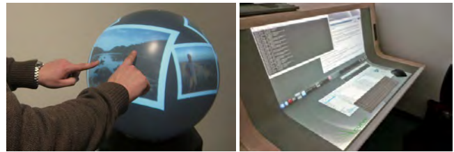
Fig. 1. a) Sphere: 360 degree multi-touch user interface for multiple access [5]. b) Curve: Continuous curved interactive desktop environment [39]
