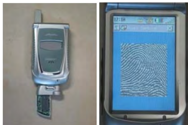
Fig. 6. Prototype of a fingerprint-sensor attached to a mobile phone. Used by Su et al. [38]
