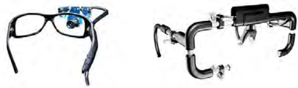
Fig. 5. Camera Eye Tracker [17] and EOG Eye Tracker [5].
