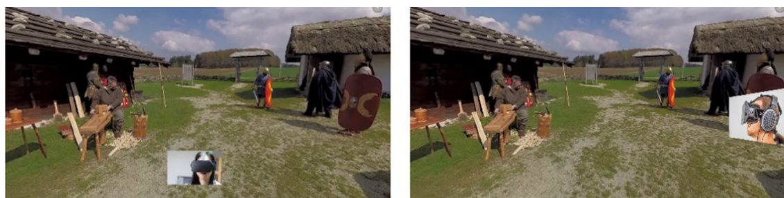
(a) Front -method: Chat window in front of the viewer, connected to the display. The co-watcher is always centered in the FoV.
