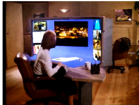
Figure 2. The digital desk shown in Tognazzini's Starfire concept video from 1994 offers a horizontal and a vertical interactive surface [27].
