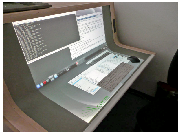
Figure 1. Curve is a digital desk concept that blends a horizontal and a vertical interactive surface. Its design takes into account existing ergonomics research and own experimental findings.
