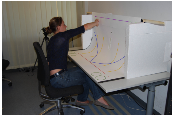
Figure 4. Arrangement of the paths on one of the paper screens. Proband of the user study had to draw these paths with one or two fingers. This task had to be performed on each of 18 prototypes. Traces enhanced for print.
