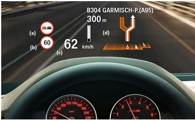
Fig. 1. BMW head-up display including information about (a) no passing-zone, (b) speed limit, (c) current speed and (d) navigation directions [4]
