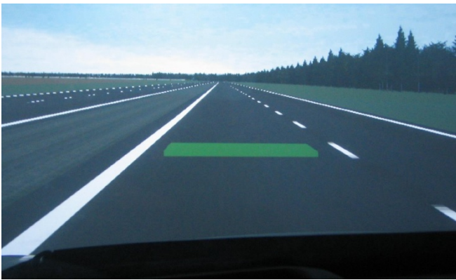
Fig. 2. Continuous braking bar in front of the vehicle.
