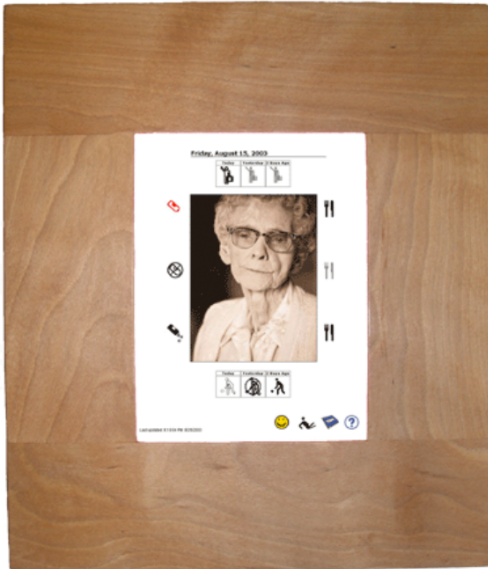
Fig. 3. The CareNet Display main overview is showing the status of the elderly supervised person by coloured icons [3]
