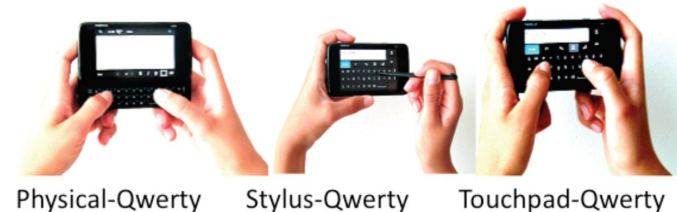
Fig. 8. Text-entry methods in Study 2. In unconstrained situations the Physical Query performed best, in constrained situations the Touch-Query was better usable [21].
