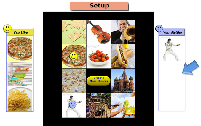
Fig. 3. Preference-based fallback authentication (setup phase) [2]. When the user clicks on "Give me more choices", all images not currently being selected are marked as Don't care and can be used as fillers during fallback authentication.
