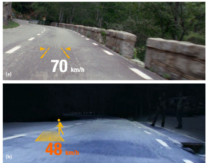
Fig. 2. Two implemented features of BMW head-up displays: (a) lane keeping warnings, (b) person detection as part of the "night vision" system [4]
