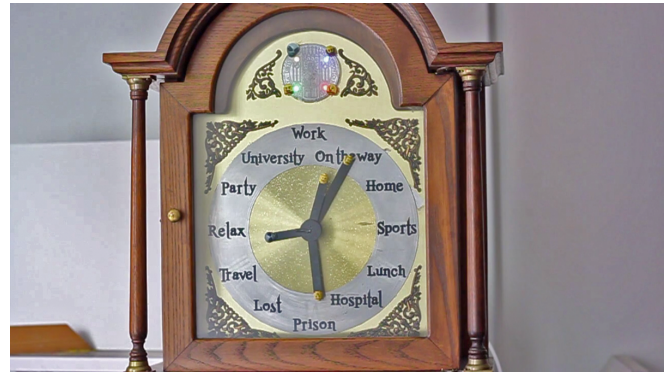
Fig. 5. Magic Clock face with multiple watch hands indicating each the current location of one person [2]
