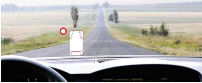
Fig. 4. Bird's eye view showing the position of imminent danger.
