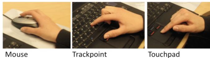
Fig. 7. Input devices in Study 1. To perform in a multitasking scenario it is easier to use Touchpad and Trackpoint than a Mouse [21].
