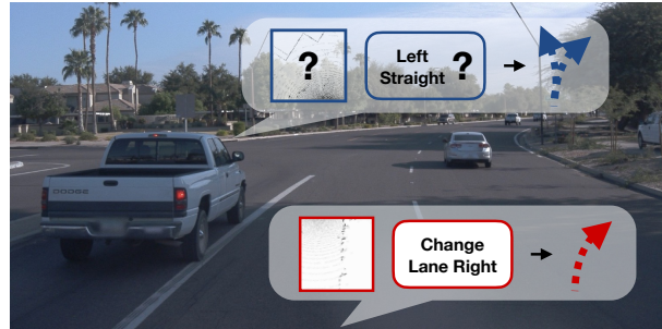
Figure 1. We present LAV, a mapless, learning-based end-to-end driving system. LAV takes as input multi-modal sensor readings and learns from all nearby vehicles in the scene for both perception and planning. At test time, LAV predicts multi-modal future trajectories for all detected vehicles, including the ego-vehicle. Picture credit – Waymo open dataset [41].
