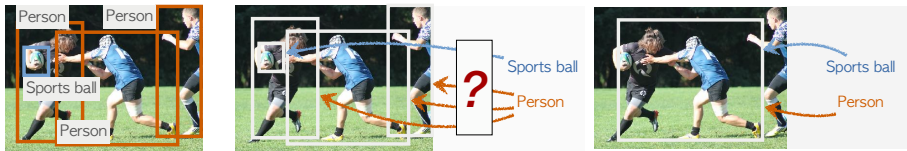
(a) Standard detection (b) Prediction-based label assignment (c) Our non-prediction-based loss Fig. 2: Left: Standard detection requires ground-truth labeled boxes and cannot leverage image-level labels. Center: Existing prediction-based weakly supervised detection methods [3, 44, 45] use image-level labels by assigning them to the detector’s predicted boxes (proposals). Unfortunately, this assignment is error-prone, especially for large vocabulary detection. Right: Detic simply assigns the image-labels to the max-size proposal. We show that this loss is both simpler and performs better than prior work.
