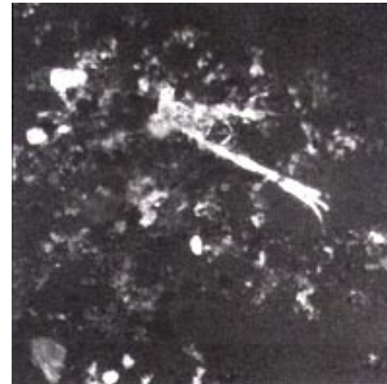
Figure 17 Left: Ferrogram of an oil sample taken from an overhauled 1200-kW, turbine-driven reduction gearbox after five days of operation. Right: Ferrogram from an oil sample from the same gearbox after one month of operation.
