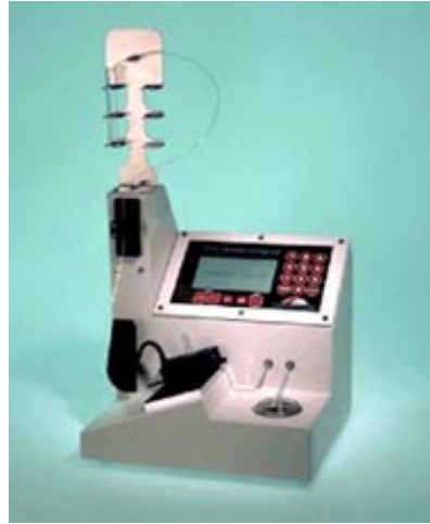
Figure 1 The DR-V Ferrograph™, a direct reading ferrograph, measures the concentration of wear particles.
