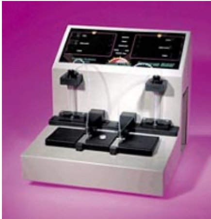
Figure 3 The FM-III Ferrograph, an instrument in the analytical ferrograph system, prepares ferrograms for analysis.
