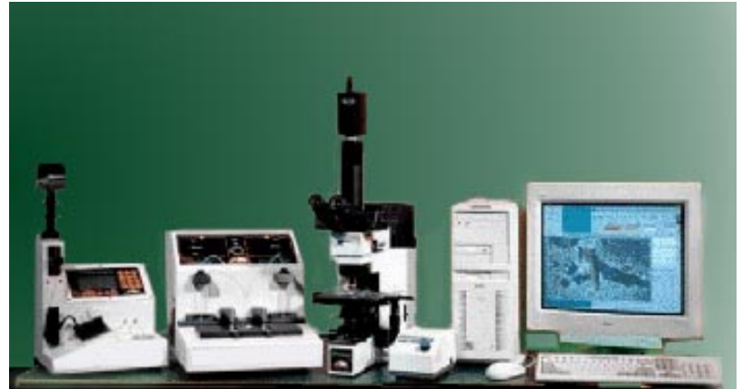
Figure 5. The PASSPORT analytical system features a video camera attached to the ferroscope. The image is sent through a computer to a video monitor.
