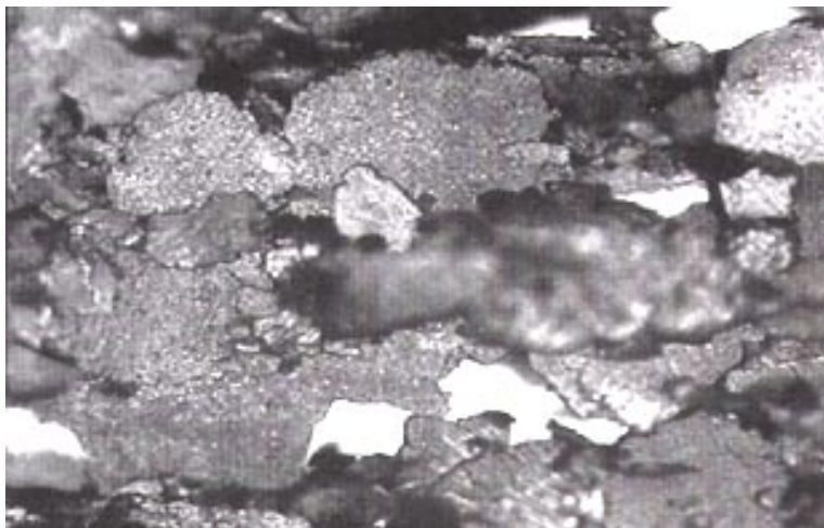
Figure 21 These wear particles indicate severe gear wear generated at the pitch line.
