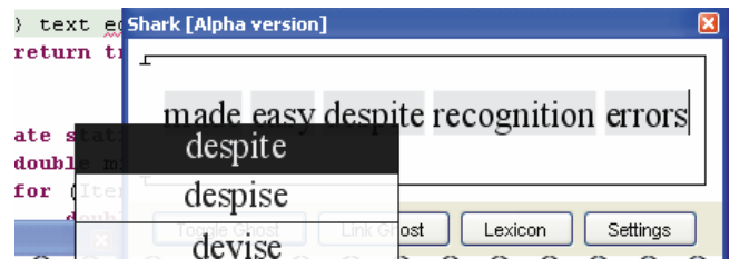
Figure 4. The stream editor showing a fragment of the sentence "Text editing made easy despite recognition errors". Gray words indicate that the user can press the stylus on them and reveal an N -best list of other possible candidate words.
