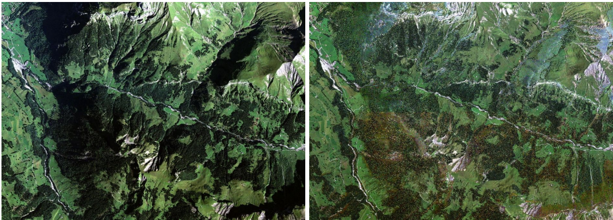
Figure 10.8: Effect of combined topographic / cast shadow correction: left: original RGB image; right: corrected image (data source: Leica ADS, central Switzerland 2008, courtesy of swisstopo).
