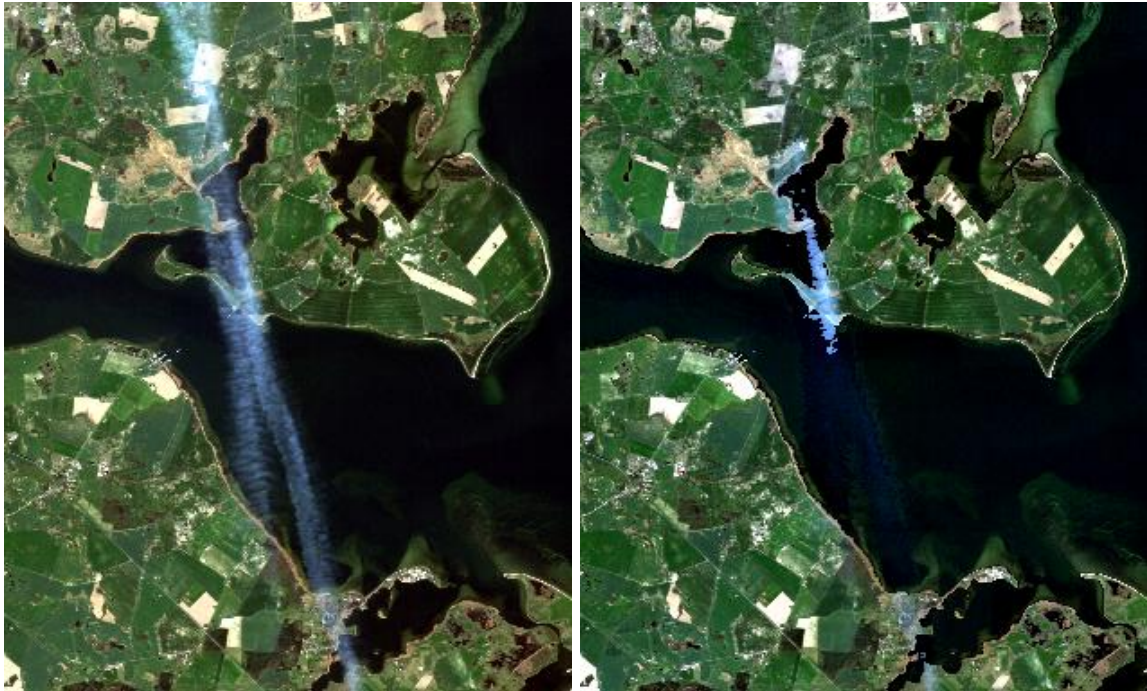
Figure 10.19: Haze removal over water, ALOS-AVNIR2 true color image, northern Germany, 16 April 2007. Left: part of original scene, right: after haze removal.
