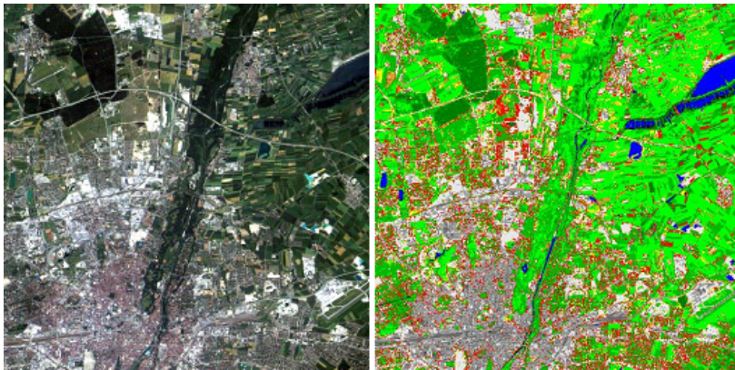
Figure 5.74: Example of classification with SPECL. Left: true color image of Landsat TM, right: result of classification.
