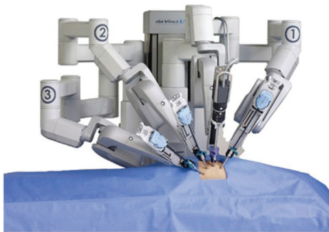
Fig. 10. Da Vinci robot used now routinely in clinical surgical procedures (Adapted from [3])
