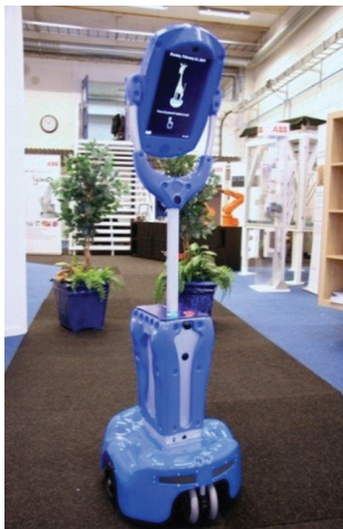
Fig. 7. HeadThere telepresence Robot tilting his display. (Adapted from [1])
