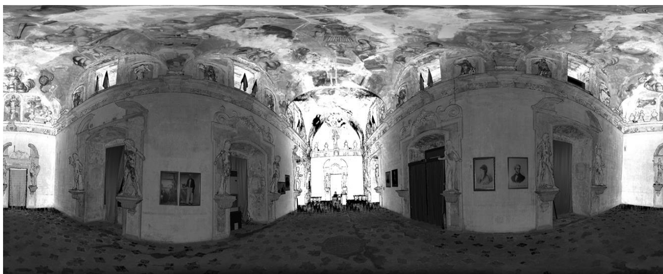
Fig. 8: Plane development of a hemispheric 3D scan
