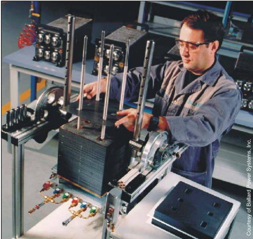
Figure 4-21 Assembling a PEM Fuel Cell Stack
