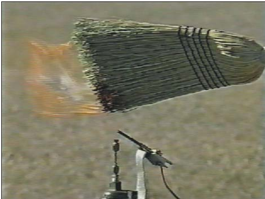
Figure 1-8 Invisible Hydrogen Flame Igniting Broom
