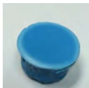
Coupons Showing Punch-Through at Inner Wall
