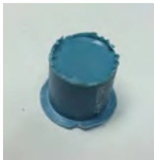
Coupons Showing Crown at Outer Surface
