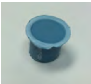
Coupons Showing Punch-Through at Inner Wall
