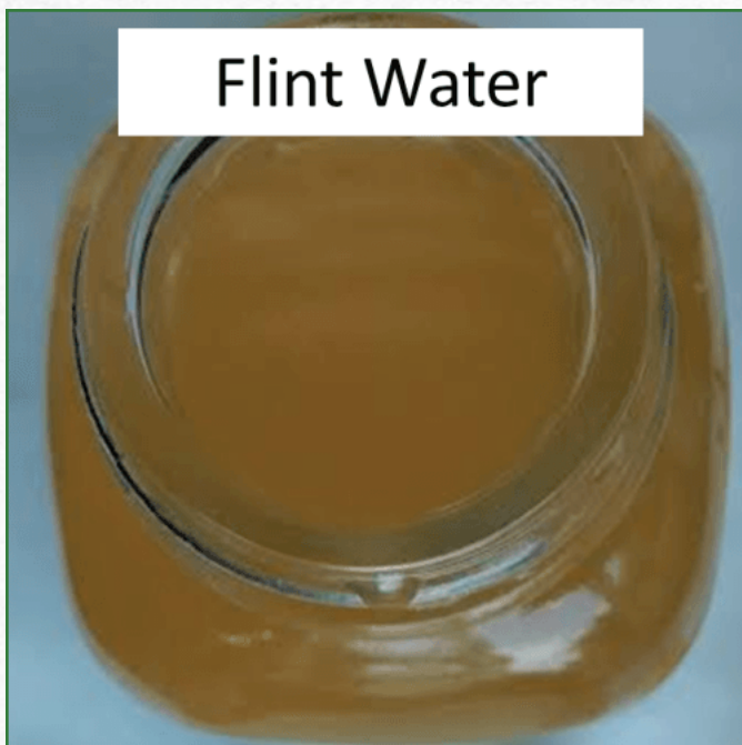
FIGURE A.24 : IRON CORROSION CAUSES "RED" OR RUSTY WATER
