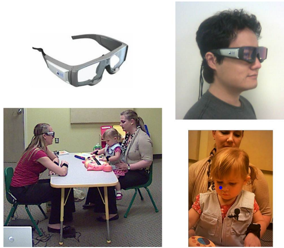
Figure 1. Experiment setup of our method. The examiner wears the SMI glasses and interact with the child (bottom left). The glasses are able to record the egocentric video with the gaze data (bottom right).
