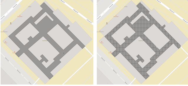
Figure 3: Floor plan of the Sennott Square building at the University of Pittsburgh campus (left) converted to a Building Grid Layout (right).
