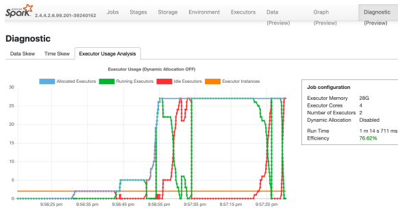
Figure 6: Executor usage with AutoExecutor as seen on diagnostic panel of an Azure Synapse Spark pool.
