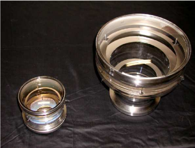
Figure 2: The 5'' (left) UV HPD and the 10'' bialkali HPD (right); the two tubes mount the same sensor and readout electronics.
