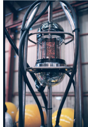
Figure 8: A 6-faced LED beacon is housed on a pressure-resistant glass cylinder fixed to the mechanical frame of an ANTARES storey.
