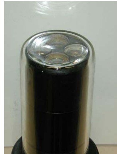
Figure 10: Implementation of the 4 PMTs in the centre of the HPMT
