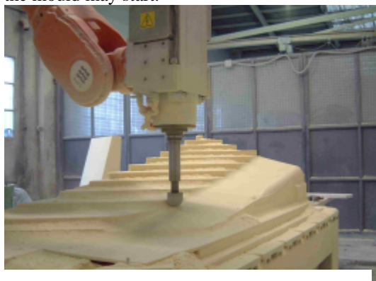
Figure 8 - Model Machining with 7-axis robot
