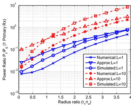
Fig. 4. Sum transmission power of one or 10 secondary transmitters under various distances and 1 primary receivers.
