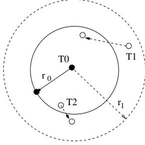
**Fig. 2.** Secondary spectrum access network: a cell with primary users (one base station T0 and  $M$  primary receivers), and secondary users ( $L$  secondary transmitters T1, T2,  $\dots$ , and their secondary receivers). Primary receivers are located within a distance of  $r_0$  to T0, whereas secondary transmitters are within a distance of  $r_1$  to T0.
