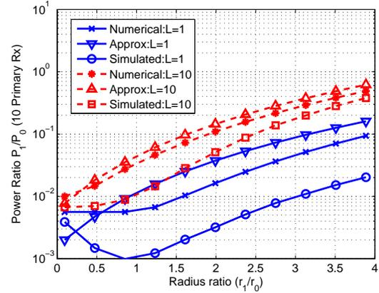
Fig. 5. Sum transmission power of one or 10 secondary transmitters under various distances and 10 primary receivers.
