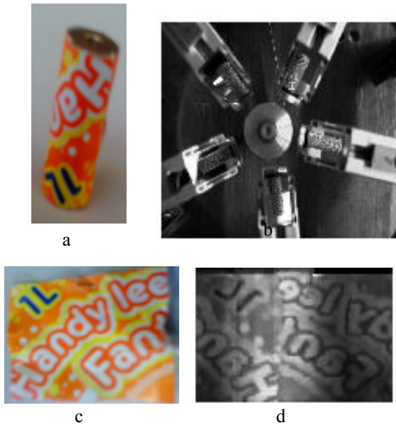
Fig. 15. (a) Pattern of letters covered cylindrical object. (b) Image from matrix camera with multiple flat mirrors. (c) Cover of the object before supporting on object. (d) Collecting of partial views after image processing.
