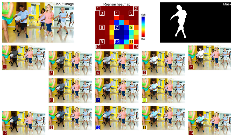
(a) A heatmap visualizes the realism score achieved when we change the estimated saturation (x-axis) and exposure (y-axis). Our estimated values (center of the heatmap) achieve the optimal realism while changing the parameters in any direction reduces the realism. Sample edited images and their corresponding location in the heatmap are also visualized.
