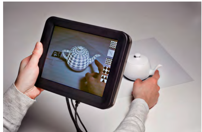
Figure 1: The user feels virtual tactile textures on a real object while observing them on a AR display. Note, that the object is not instrumented with any tactile actuation apparatus.
