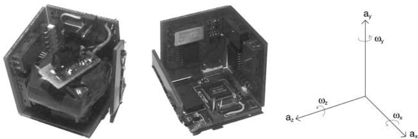
Fig. 1. Current IMU hardware and reference frame
