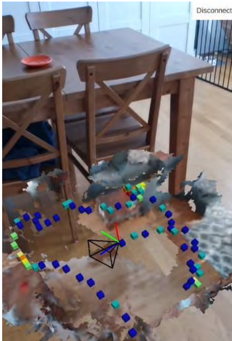
Figure 80 - Augmented reality radiation measurement real-time visualization screenshot (seen from third-person perspective with environmental meshing) (5)
