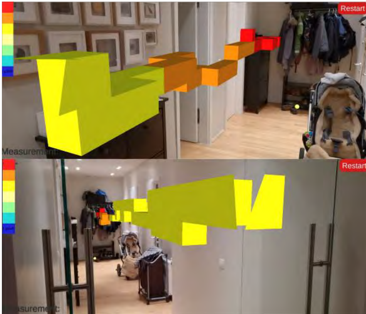
Figure 110 - Example of advanced AR approach showing virtual measurements taken in real-time locked in the environment from two different angles
