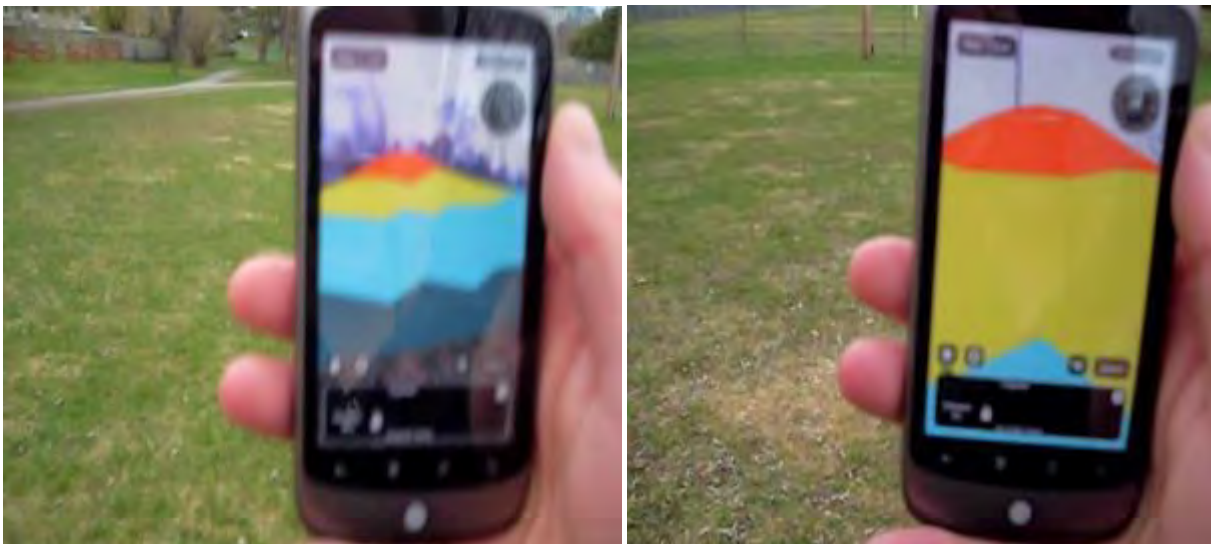
Figure 37 - Real-time visualization of point source 3d mesh in AR interface via Layer Reality Browser (seen as approaching)
