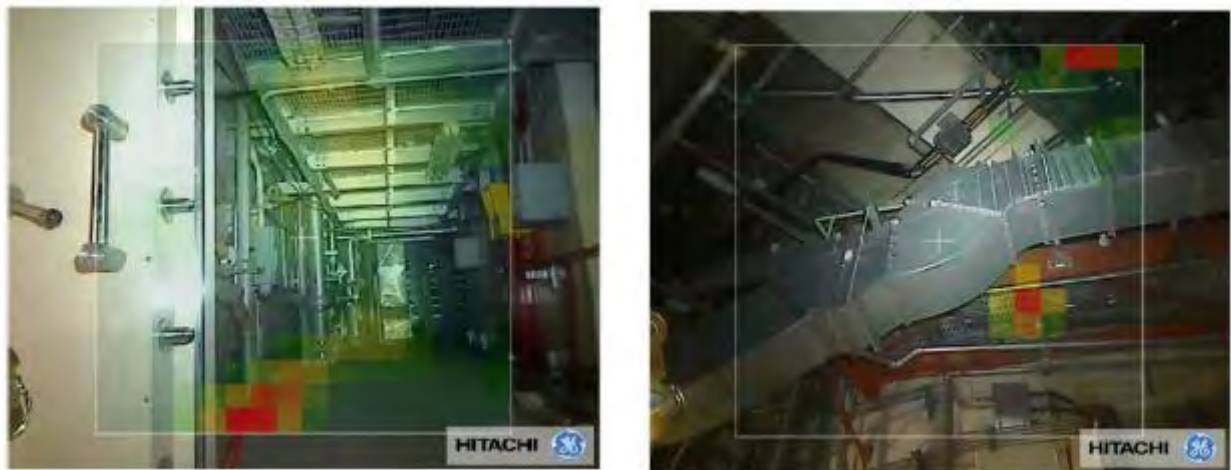
Figure 2 - Example of robot survey with gamma camera survey taken inside Reactor Building for Unit 1 at the Fukushima Daiichi NPS[28]
