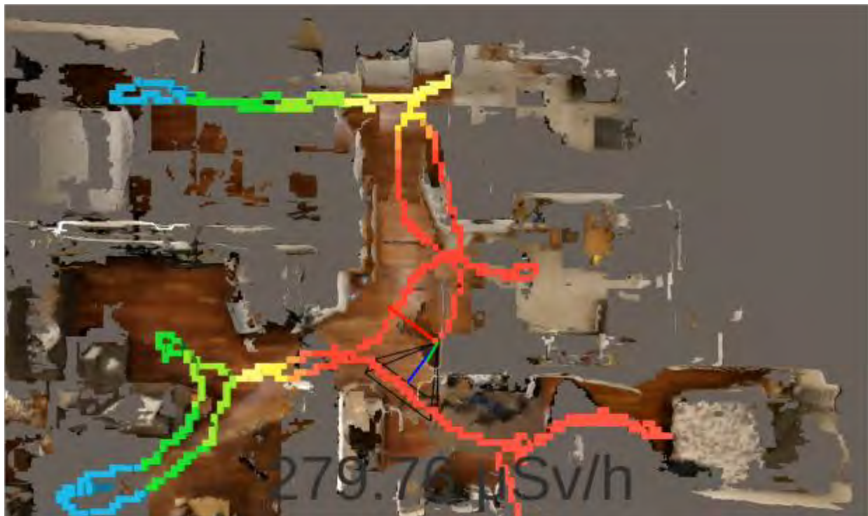
Figure 108 - Example of advanced AR approach showing a top down perspective helping the user understand where the source may be located
