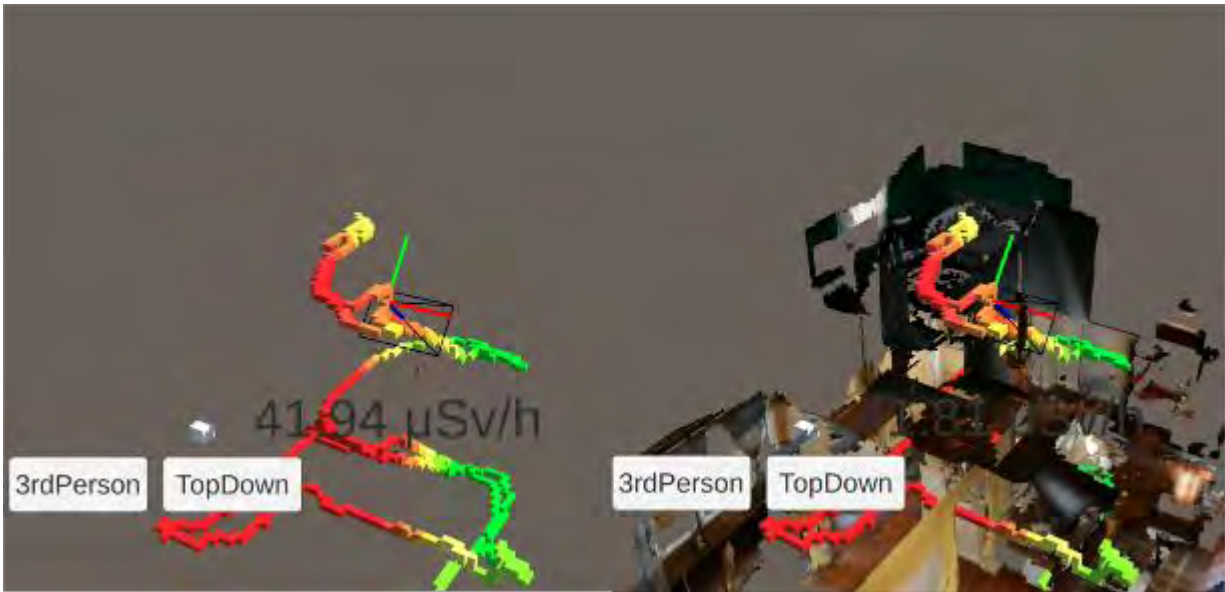
Figure 106 - Example of advanced AR approach showing the benefits of real-time meshing to help contextually understand where measurements are being taken in the environment
