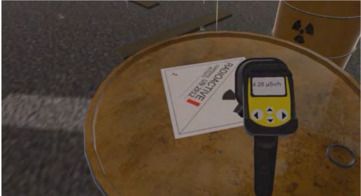
Figure 90 - Screenshot from the transport accident with radiological material in severe weather with showing the user investigating a drum, visually inspecting its signage, conditions and taking radiation measurements
