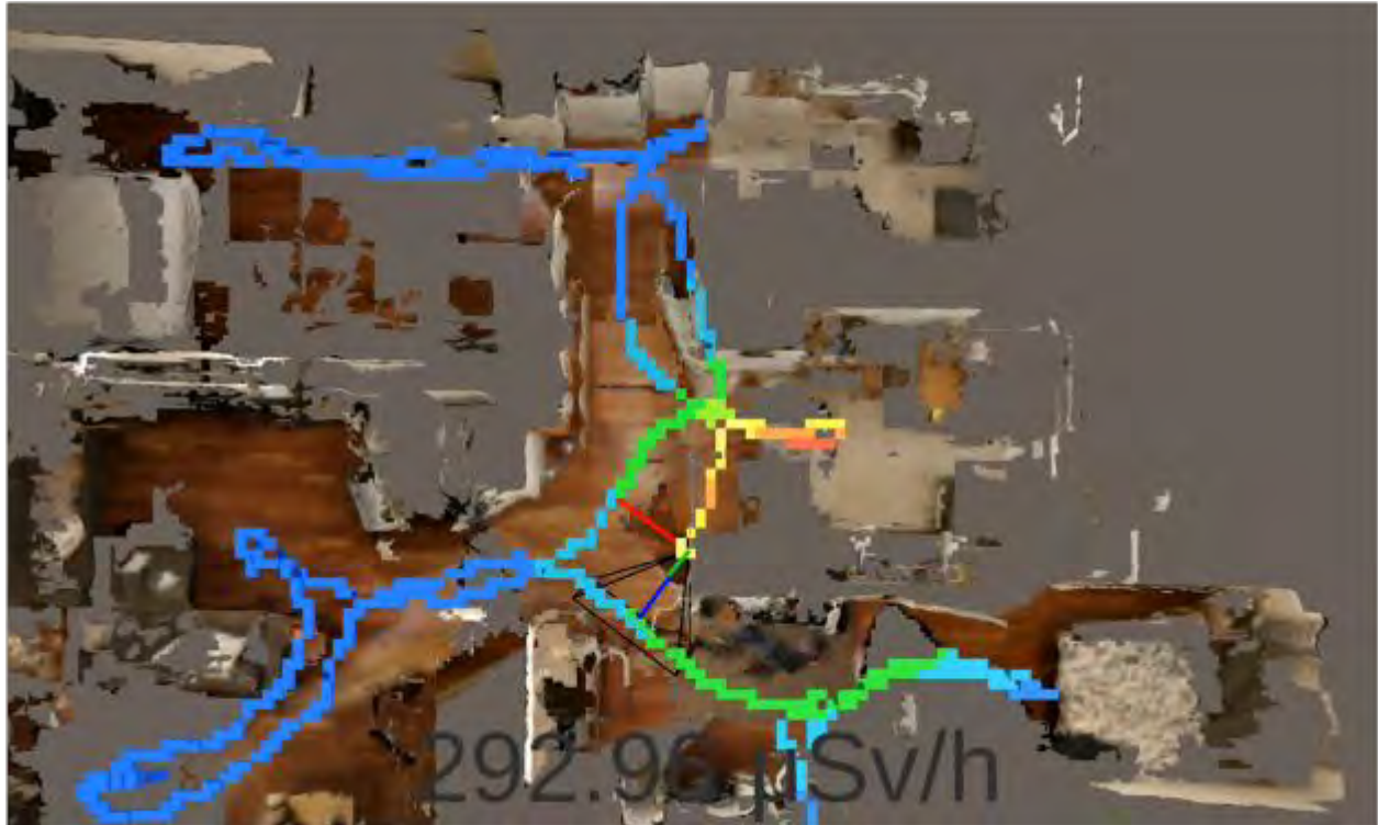
Figure 109 - Example of advanced AR approach showing a top down perspective helping the user understand where the source may be located with a modified scale to more clearly indicate the highest locations
