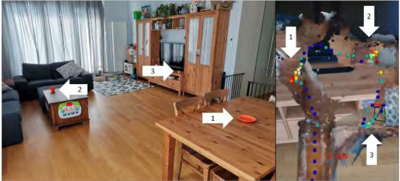
Figure 112 - Example of advanced AR approach showing measurements of three sources from top-down angle with environmental meshing
