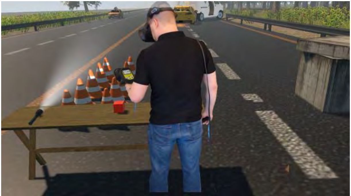
Figure 99 - User beginning a scenario picking up a radiation detector from a table and examining its response with a check source (filmed in mixed reality)
