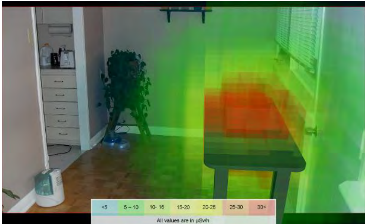
Figure 11 - Point source on a table with scale (isometric perspective) and 3d visualized radiation field
