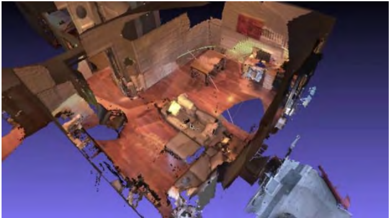
Figure 45 - Preliminary environmental scan taken with included Tango constructor application (highlighting detail captured in close range)
