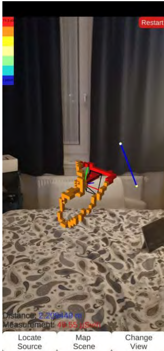
Figure 118 - Third person perspective of measurements and a guess (white sphere) 2.20 m (blue line) from actual source (yellow sphere)
