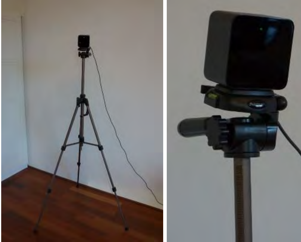
Figure 14 - HTC Vive base station mounted on camera stand (only one visible) and close-up
