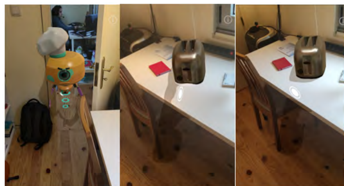
Figure 24. Shadow projection limitations using DepthLab: shadows are only partially displayed and cross surfaces.
