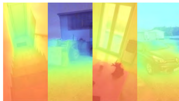
Figure 4. Depth data estimated from monocular views (closer surfaces in red and surfaces further away in blue).
