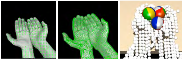
Figure 8: Depth aware optical flow. Left: Flow field computed from RGB image. Middle: Tracked particle positions. Right: Physics particles interacting with virtual spheres.
