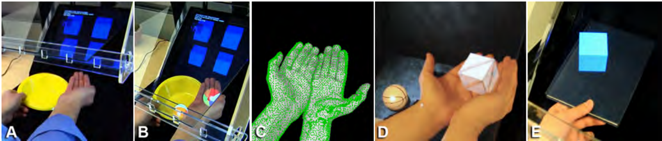
Figure 1: HoloDesk allows direct freeform interactions with 3D graphics, without any body-worn hardware. A + B) User sees a virtual image of a 3D scene through a half silvered mirror. Scene is corrected for the viewer's perspective. User can freely and directly reach into the 3D scene to interact with it. C + D) A novel algorithm is presented that allows diverse and unscripted whole-hand 3D interactions e.g scooping and grasping. E) Other real objects beyond hands can be used for interaction.
