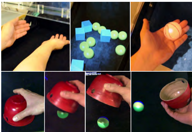
Figure 3: Top: User's hands in the interaction area. 3D scene as seen by the user. Virtual sphere resting on hand. Bottom: Real object occludes virtual, casts shadows.
