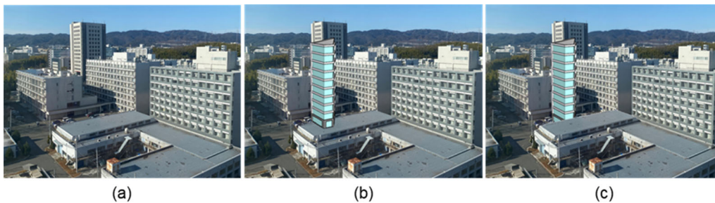
Figure 1 Occlusion problem in AR (a) Real world (b) AR with incorrect occlusion (mock-up) (c) AR with correct occlusion (mock-up)
