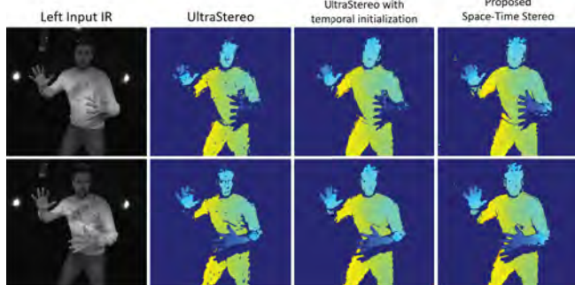
Fig. 13. Qualitative comparisons with UltraStereo [Fanello et al. 2017b], and a variant of this method including the initialization from Sec. 5.2. Notice how the proposed space-time stereo provides more complete disparity maps in low SNR regions (e.g. hair) as well as in slanted regions.
