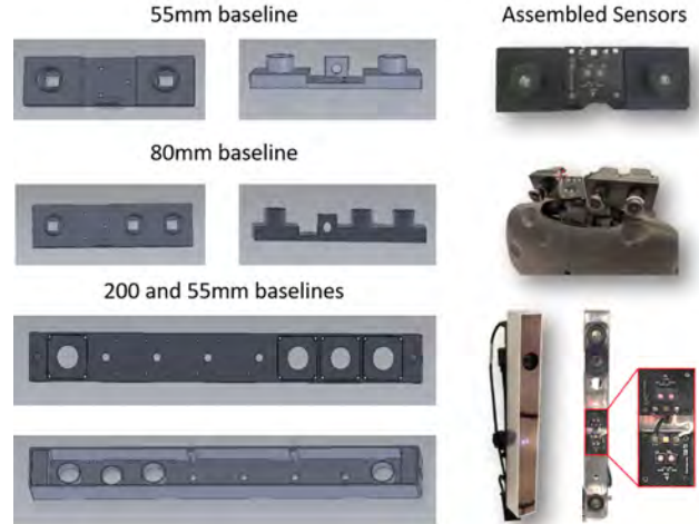
Fig. 3. (left) In the additional materials we provide CAD fabrication models for our active stereo camera systems at different baselines. (right) The 55mm baseline for exo-centric short range interaction (depth only), 80mm baseline for ego-centric VR headsets (depth+RGB) and hybrid 200mm/55mm for long range (full body, depth+RGB) capture.
