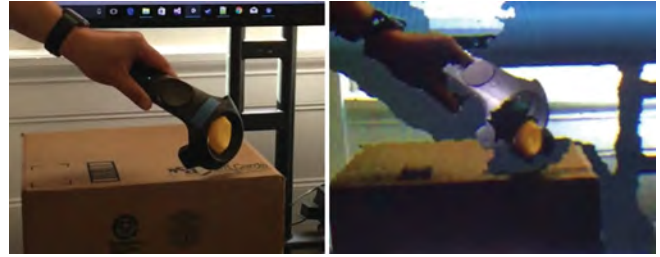
Fig. 20. Frame-by-frame motion trajectory and latency analysis. Left: direct slow motion capture of a HTC Vive controller with a physical target. Right: slow motion capture of depth rendering through the HTC Vive VR headset.
