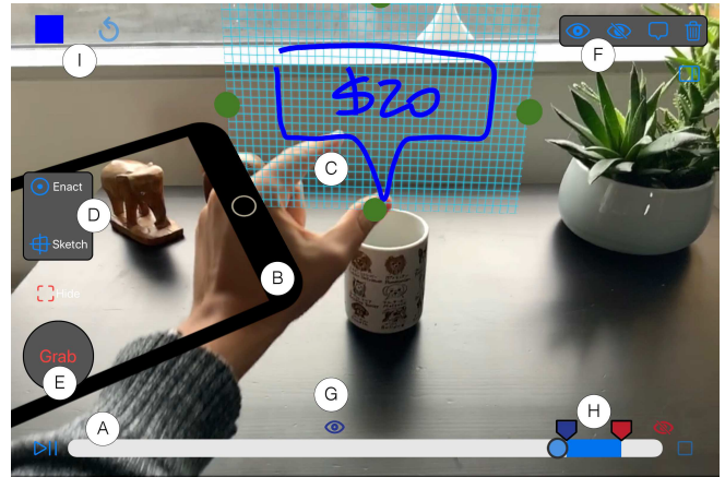
Figure 2. PRONTO's playback screen: (A) The timeline can play/pause the recorded video shown in the background, (B) a visualization of the current tablet's position, (C) a spatial layer with a sketch, (D) the "Sketch" button creates new spatial layers at the tablet's position, (E) the "Grab-Drop" moves the selected spatial layer by moving the tablet, (F) the selected layer can appear/disappear/face the camera or be deleted, (G) the timeline shows when the selected spatial layer appears/disappears, (H) and the selected animation beginning and duration, (I) undo and stroke color.
