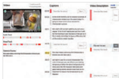
Figure 1: Our system (A) identifies accessibility issues by locating modality asymmetries (in red) between audio segments and video segments using cross-modal grounding. (B) lets authors address accessibility issues using the CrossA11y interface to write captions and video descriptions, and (C) creates a more accessible video from the authored descriptions.
