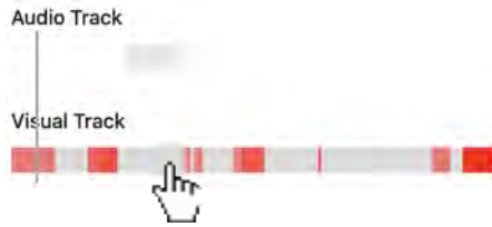
Figure 3: Authors can hover on segments of visual/audio timelines in CrossA11y to inspect the computed correspondence between the selected segment and segments in the other modality. Here, opaque segments in the audio track are the segments predicted by the system to match the segment in the video track.
